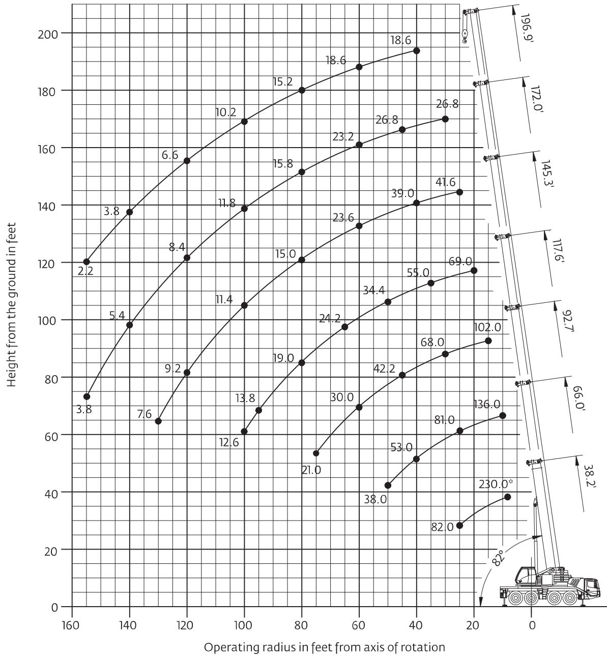
*Hook heights shown in the working range diagram do not consider loaded boom deflection.*
