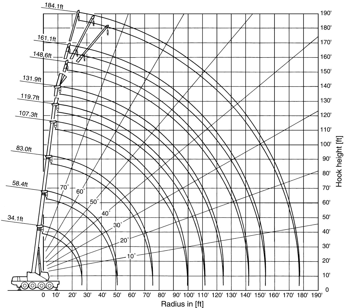
**NOTE:** Boom and jib geometry shown are for unloaded condition and machine standing level on firm supporting surface. Boom deflection and subsequent radius and boom angle change must be accounted for when applying load to hook.
