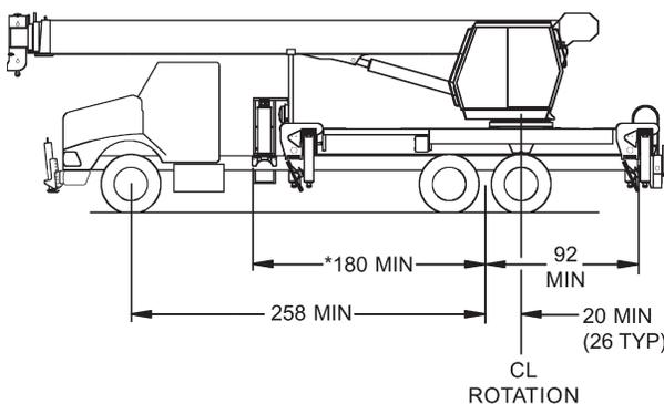
\*CLEAR OF OBSTRUCTIONS (MUFFLERS, EXHAUST STACKS, ETC.) ON TOP OF TRUCK FRAME FOR FULL 8 FOOT (2.44m) WIDTH.
