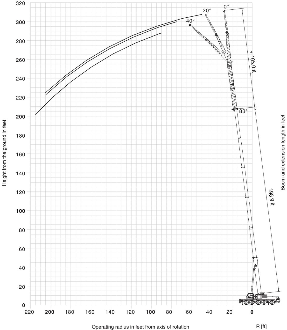
Hook heights shown in the working range diagram do not consider loaded boom deflection.
